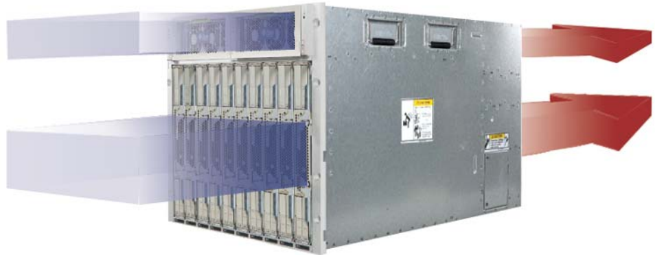
Figure 4. The Sun Blade 6000 Modular System uses strict, front-to-back cooling and two separate airflows.
