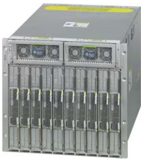
Figure 1. The Sun Blade 6000 Modular System supports up to 10 server modules in only 10 rack units.
